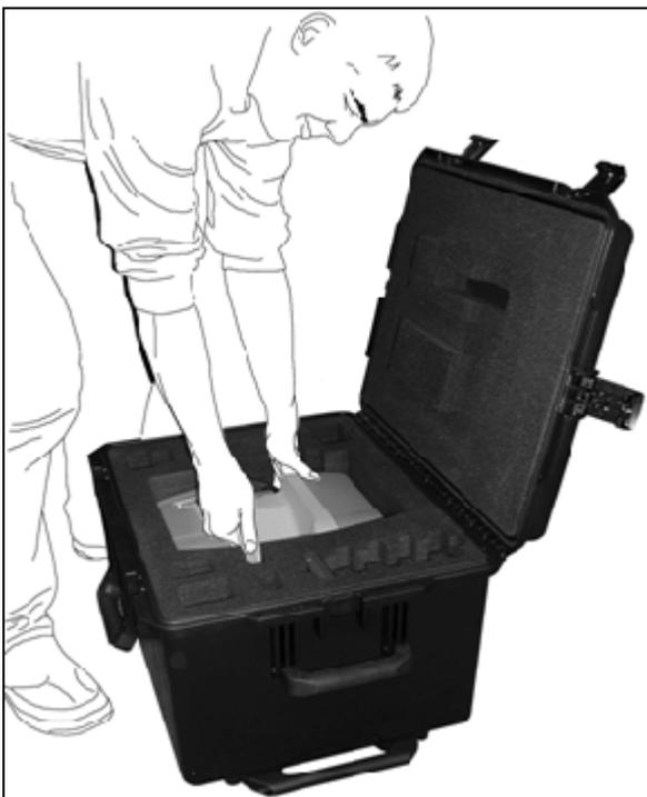
5. Lift the instrument assembly out of the case:
