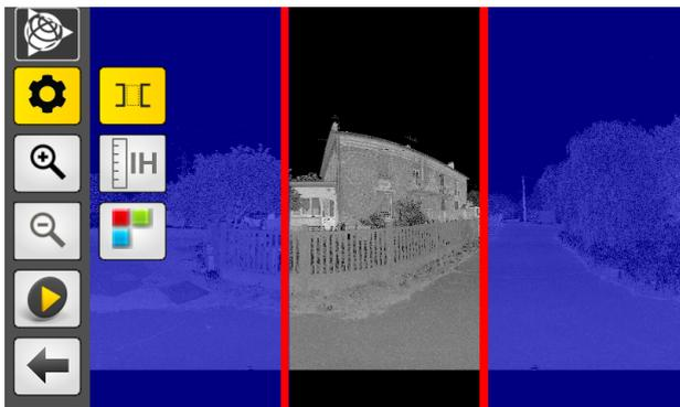
The default size of the scan area is one-third the size of the Full scan display. Areas that are shaded blue are not scanned.
