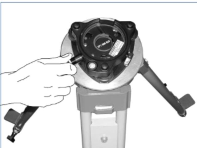
3. Look again through the optical plummet eyepiece. If the cross-hairs are not exactly over the control point on the ground, do one of the following:
